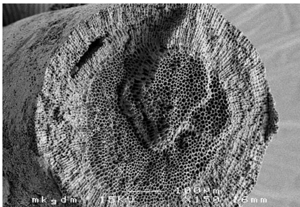
Fig 13-12 Three-dimensional morphological structure of the calcite skeleton of the raw algae is maintained from the beginning through to production of the final material (190x; white bar, 100 \mu m).
